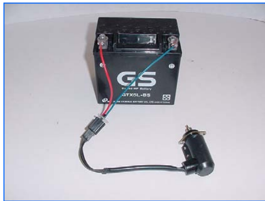
12 volts applied to the choke cylinder
